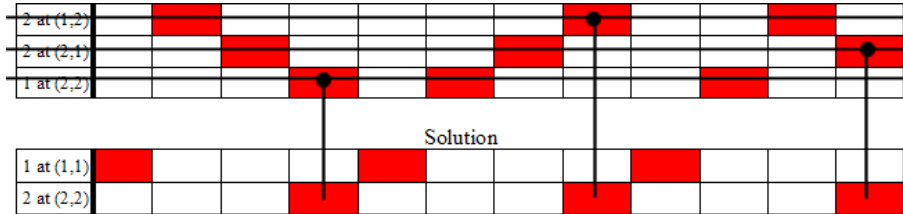
Figure A.4: Step 4: Add row to solution set and delete all conflicting rows.
